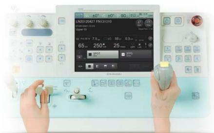
The high-speed dual processing system can simultaneously process images, register patient information, or perform other tasks quickly in real time, without interfering with examinations.
